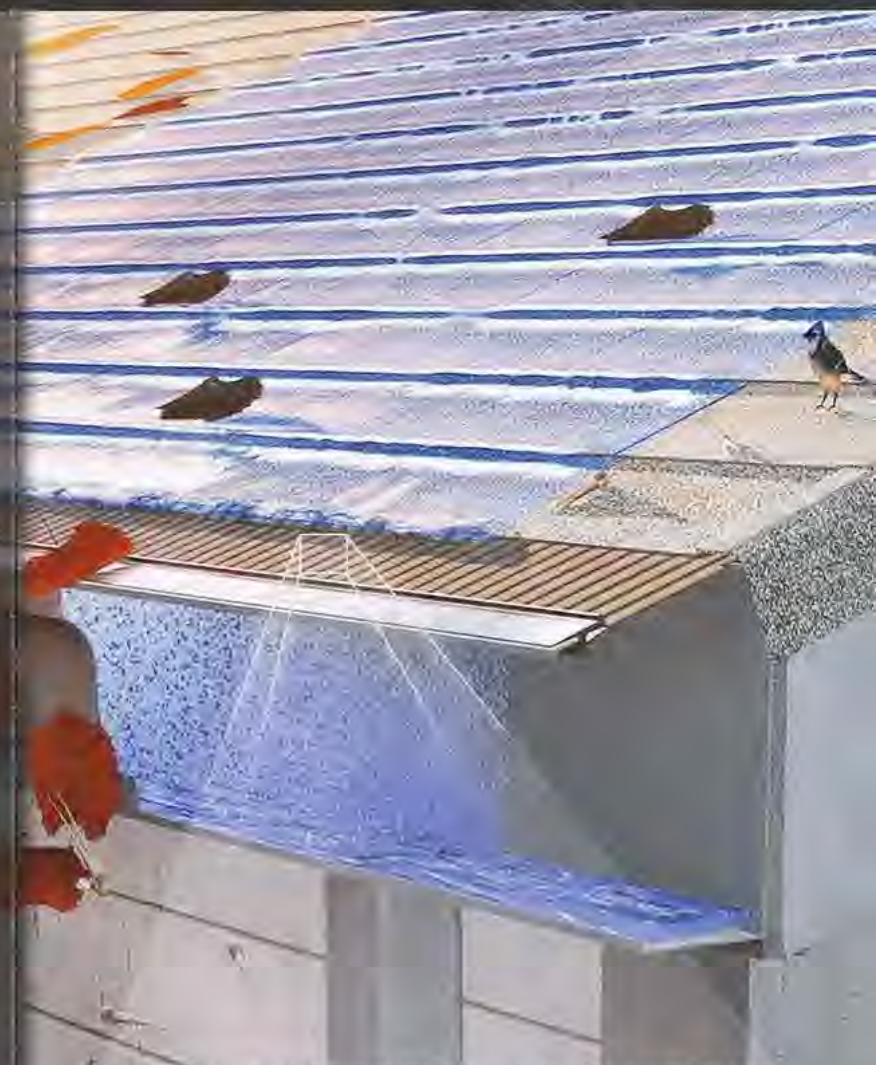
The conveyance tube is slanted towards the rainwater collection tanks so the tanks can fill up with clean fresh rainwater.
